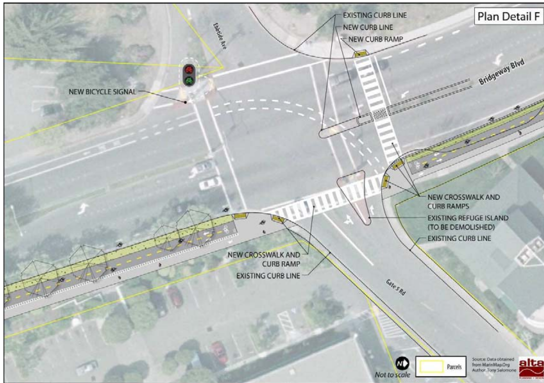
Figure 7-51 Gate 5 Road Intersection Improvement Option - Bike Signal
